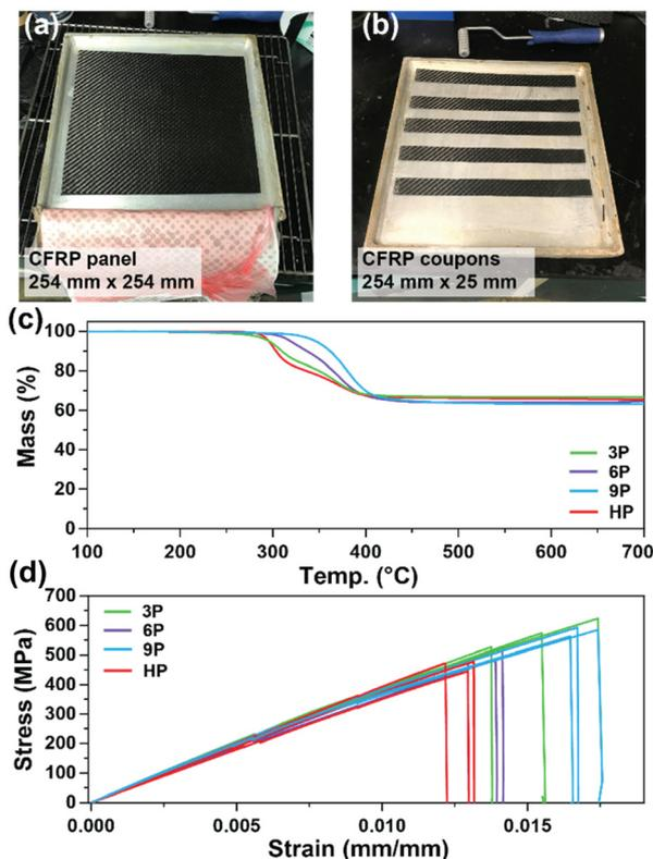
**Fig. 4** (a and b) Photos of CFRP composite panel (254 mm × 254 mm) prepared and cut (25 mm × 254 mm) for mechanical testing. (c) Thermogravimetric analysis to determine resin-to-fiber ratio after composite cure and processing. (d) Stress–strain curves for CFRP composites.
