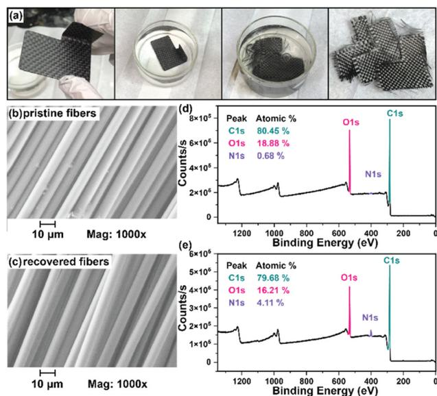
**Fig. 8** (a) Degradation of a 6P CFRP laminate part *via* submersion in 1 M HCl showing full dissolution of the polymer matrix and separation of carbon fiber layers after washing with DI water and drying. SEM of (b) pristine carbon fibers and (c) carbon fibers recovered after polymer thermoset hydrolysis. XPS survey analysis of (d) pristine and (e) recovered carbon fibers.
