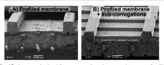
Fig. 15 Images obtained from a scanning electron microscope for (A) the profiled membranes (B) and profiled membranes with subcorrugations (figures and captions reproduced from ref. 193 with permission from Elsevier, copyright 2014).
