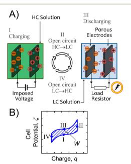
Fig. 20 (A) Illustration of the working principle of capacitive energy extraction based on double layer expansion (CDLE) and (B) the qualitative plot of useful work W produced in an unit Capmixing cycle (figures and captions reproduced from ref. 69 with permission from American Chemical Society, copyright 2016).
