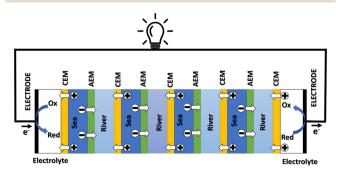
Fig. 14 A schematic illustration of the RED process.
