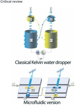
Fig. 1 Top, classical Kelvin water dropper, bottom, representation of the microfluidic version (figures and captions reproduced from ref. 16 with permission from Royal Society of Chemistry, copyright 2013).
