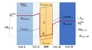
Fig. 13 Schematic representation of concentration, c, and potential,  $\phi$ , profile in the bulk solutions, the stagnant diffusion layers (SDLs), and in an ion exchange membrane (IEM) (figures and captions adapted from ref. 164 with permission from FIMTEC & MPRL, copyright 2016).
