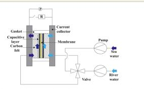
Fig. 22 Scheme of the experimental millifluidic set up used for the salinity gradient harvesting with one membrane and a 6 mm water compartment (figures and captions reproduced from ref. 169 with permission from Elsevier, copyright 2022).
