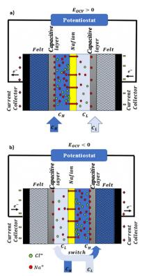
Fig. 23 Illustration of two working regimes for a capacitive salinitygradient cell before (a) and after (b) water compartment switch (figures and captions reproduced from ref. 169 with permission from Elsevier, copyright 2022).
