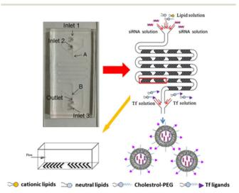
Fig. 7 Schematic representation of Tf-LNP fabrication using the staggered herringbone micromixer. Reprinted with permission from ref. 99. Copyright 2016. Elsevier.
