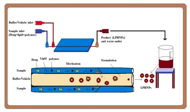
Scheme of the setting of the microfluidic apparatus and of the LPHNS fabrication. Reprinted with permission from ref. 125. Copyright 2020. Elsevier.
