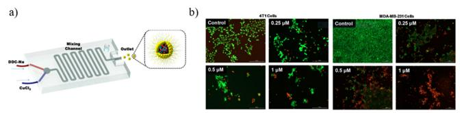
Fig. 16 (a) Schematic illustration of the mixing microfluidic device adopted to fabricate BSA/Cu(DDC)<sub>2</sub> MONPs. (b) MTT assay results of 4T1 cells and MDA-MB-231 cells treated with BSA-Cu(DDC)<sub>2</sub> for 48 hours. Reprinted with permission from ref. 162. Copyright 2019. Elsevier.
