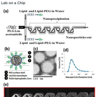
Fig. 11 Nanoprecipitation of lipid-polymeric NPs: (a) schematic representation of Tesla structures for the production of hybrid lipidpolymeric NPs, (b) figure of a NP. (c) TEM image of NPs, (d) average size distribution of NPs  $d \sim 40$  nm. (e) Solvent mixing in the Tesla micromixing structures with a scale bar of 100 µm. Reprinted with permission from ref. 129. Copyright 2010. American Chemical Society.
