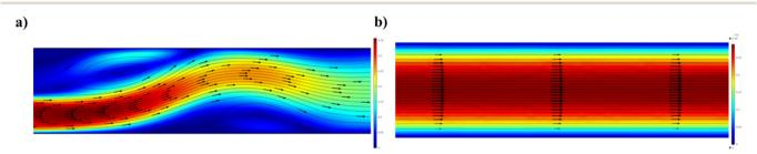
Fig. 1 Schematic illustration of different types of representative flow patterns in FEM microchannels simulated using COMSOL Multiphysics® (velocity magnitude (m/s)); the arrows represent the streamline velocity field: a) turbulent flow and b) laminar flow.
