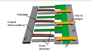
Fig. 4 Array structure of parallel polymer-based laterally amplified chemo-mechanical (LACM) unit cells. Reprinted from ref. 138 (under a Creative Commons license (CC BY 4.0)).
