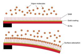
Fig. 5 Schematic diagram of a cantilever bending due to differential adsorption of analyte molecules. Reprinted with permission from reference Elsevier, 2007, pp. 109-130. 156 Copyright 2007 Elsevier.
