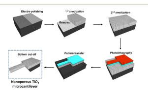
Fig. 6 Schematic illustration of the fabrication process of a nanoporous TiO<sub>2</sub> microcantilever. Reprinted (adapted) with permission from Anal. Chem., 2014, 86(10), 5077-5082.165 Copyright 2014 American Chemical Society.
