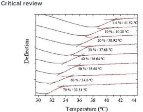
Fig. 3  $T_g$  variation (from 42 °C to 34 °C) as a function of humidity in the range between 1.4% and 70%. Reprinted with permission from reference *Polym. Test.*, 2018, **65**, 407–413. 112 Copyright 2018 Elsevier.
