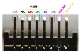
8 Optical microscopy image of the sorbent-coated microcantilever array. Reprinted (adapted) with permission from reference Environ. Sci. Technol., 2011, 45(13), 5704-5709. Copyright 2011 American Chemical Society.
