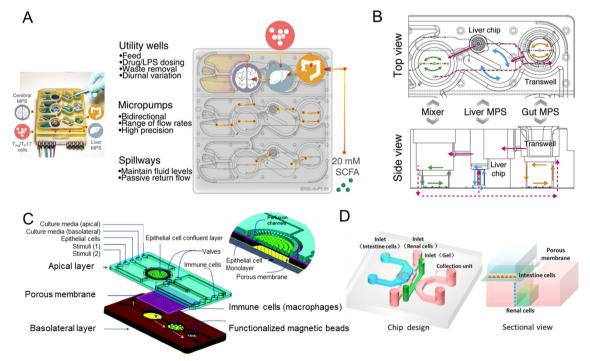
Fig. 8 Microfluidic models of the gut-x axes. (A) Design, features, and parameters of the gut-liver-brain platform. (B) Top and side view of the model of the human gut-liver axis, including adaptive immune cells. 117 (C) Schematic of the microfluidic chip forming the miniaturized gastrointestinal tract. 118 (D) Schematic of the multi-layered intestine-kidney chip. 119
