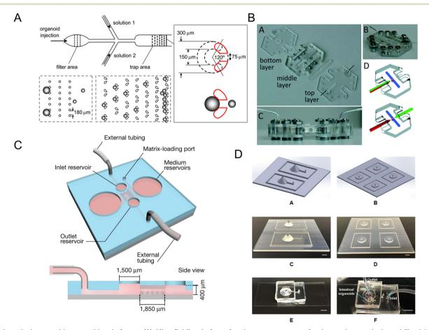
Fig. 6 Intestinal organoids-on-a-chip platforms. (A) Microfluidic platform for the measurement of volume changes in immobilized intestinal enteroids.<sup>103</sup> (B) Establishment of a gut organoid flow chip with laser-cut silicone gaskets.<sup>24</sup> (C) Schematic of a 3D hydrogel-containing microdevice developed for the culture of tubular mini-guts and dimensions of a microchannel.<sup>23</sup> (D) Scheme of long-term perfused intestinal organoids-on-a-chip with a PDMS pocket chamber. 104
