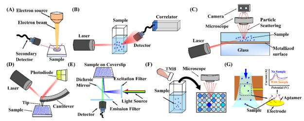
Fig. 6 Schematic representation of the working principle of nanoparticle measurement and detection techniques. (A) Electron microscopy.<sup>260</sup> (B) DLS.<sup>265</sup> (C) NTA.<sup>267</sup> (D) AFM.<sup>279</sup> (E) Fluorescence detection.<sup>286</sup> (F) Colourimetric detection.<sup>294</sup> (G) Electrochemical detection.<sup>304</sup>
