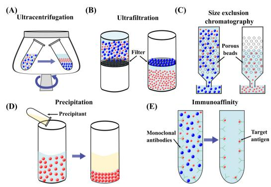
Fig. 2 Schematic diagrams of conventional techniques for submicron and nanoparticle separation. (A) Ultracentrifugation. (B) Ultrafiltration. (C) Size exclusion chromatography. (D) Precipitation. (E) Immunoaffinity capture. (17)
