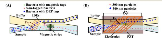
Fig. 5 Hybrid microfluidic techniques for sorting submicron and nanoparticles. (A) Sorting multiple bacterial targets by serially combining DEP and MP in an integrated DEP-MP cell sorter.<sup>251</sup> (B) A vDLD system for sorting sub-micrometre particles by coupling acoustic and DEP forces.<sup>252</sup>
