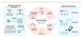
Fig. 1 Overview of microneedle-based transdermal detection and sensing devices, including biomarker/biofluid extraction strategies (left), different targets (middle), and detection and sensing principles (right).
