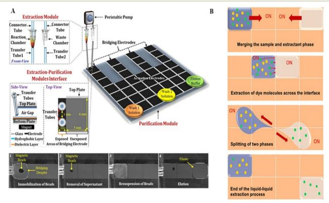
Fig. 7 DMF-based nucleic acid extraction. A) "World-to-DMF" integrated system effectively collecting target analytes based on solid-phase separation. Copyright 2014, the American Chemistry Society. B) Liquid-liquid nucleic acid extraction by handling sample droplets and immiscible extractant phases. Copyright 2021, the American Institute of Physics. 62
