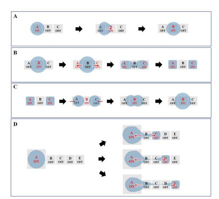
Fig. 4 Schematic diagram of manipulations on DMF including A) droplet transport, B) droplet splitting, C) droplet merging and D) droplet dispensing. The square in the figure represents the actuation electrode unit, ON means electrical potential applied to the electrode unit, OFF means switching off the electrode unit, and the arrow indicates the movement direction of the droplet.
