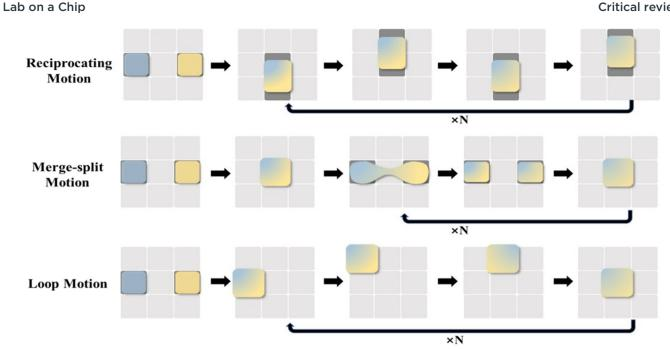
Fig. 5 Schematic diagram of droplet merging by reciprocating motion, merge-split motion, and loop motion.
