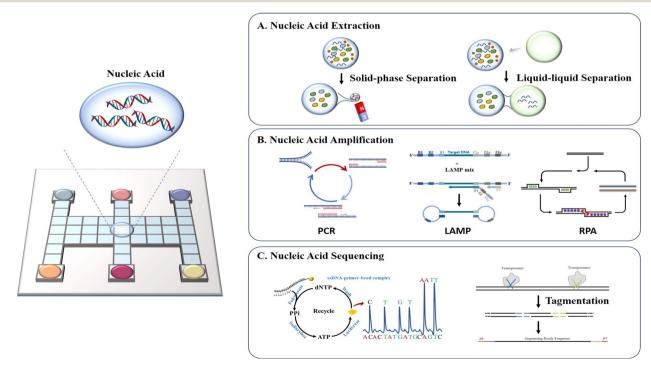
Fig. 6 Schematic diagram of DMF-based nucleic acid assays including A) nucleic acid extraction, B) nucleic acid amplification, and C) nucleic acid sequencing.
