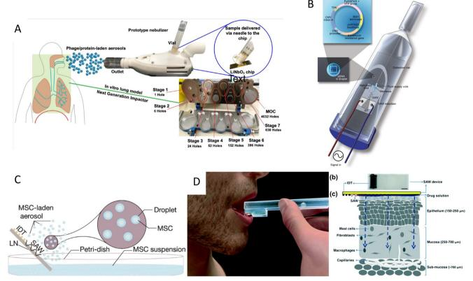
Fig. 7 Acoustic devices for drug delivery. A) Acoustic nebulization for pulmonary drug delivery of aerosols.<sup>123</sup> B) Acoustic nebulization for pulmonary plasmid delivery.<sup>36</sup> C) Stem cell delivery by acoustic nebulization.<sup>124</sup> D) Acoustic waves for permeabilization of tissue and inducing localized immune response. 125 Reprinted with permission.
