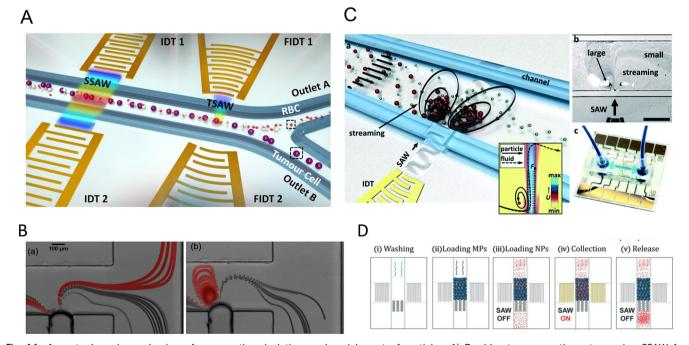
**Fig. 14** Acoustophoresis mechanisms for separation, isolation, and enrichment of particles. A) Double stage acoustic system using SSAW for alignment and TSAW for separation, <sup>224</sup> B) particle separation by microstreams from oscillatory bubbles, <sup>227</sup> C) particle separation by microstreams from focused TSAW. <sup>225</sup> D) Exosome enrichment by Bjerknes forces. <sup>238</sup> Reprinted with permission.
