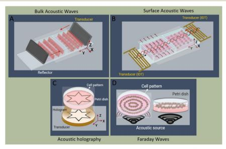
Fig. 3 Schematic of cell patterning modes, including A) bulk acoustic waves, B) surface acoustic waves, C) acoustic holography, and D) Faraday waves
