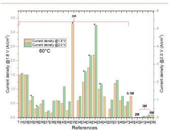
Fig. 7 Comparison at 60 °C among the values of current densities from the literature obtained at 1.8 V and 2.0 V, with different KOH concentrations. \* corresponds to cells based on noble metals at both anode and cathode.
