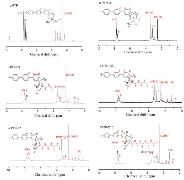
Fig. 1 <sup>1</sup>H NMR spectra of PTP (a) and various PTP-Cx polymers (b-f).
