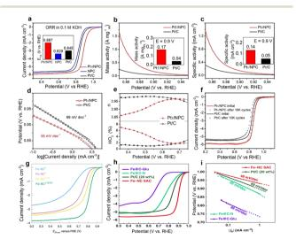
Fig. 3 (a-f) The ORR performance of single-atom platinum catalysts. Reprinted with permission from ref. 77. Copyright 2021, Elsevier; (g) The ORR activity of a single-atom Fe catalyst. Reprinted with permission from ref. 44. Copyright 2022, Springer Nature; (h and i) Steady-state ORR polarization curves and corresponding Tafel of Fe-NC SAC, Pt/C and control samples. Reprinted with permission from ref. 38. Copyright 2019, Springer Nature.
