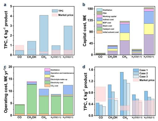
Fig. 5 (a) TPC; (b) capital cost and (c) operating cost for  $CO_2R$  to CO,  $CH_3OH$ ,  $CH_4$ , and syngas  $(H_2/CO \ (1:1) \text{ and } H_2/CO \ (2:1))$  in the base case; (d) TPC for each product in the future cases.
