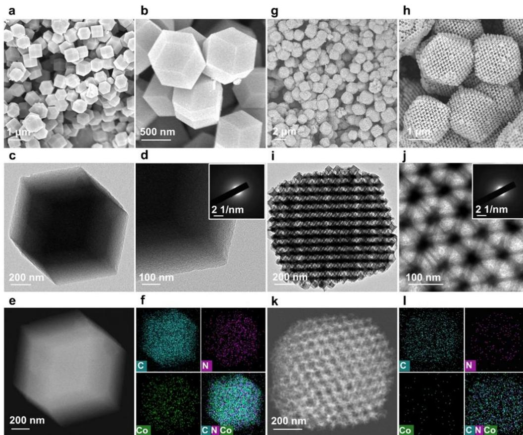
**Fig. 5** SEM images of (a and b) Co-SA/NC and (g and h) 3DOM-NC. TEM images of (c and d) Co-SA/NC and (i and j) 3DOM-NC. The insets of (d) and (j) are the SAED patterns of Co-SA/NC and 3DOM-NC, respectively. HAADF-STEM images and corresponding EDS elemental mapping images of (e and f) Co-SA/NC and (k and l) 3DOM-NC.
