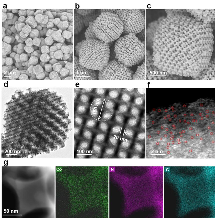
**Fig. 2** (a–c) SEM images of Co-SA/3DOM-NC at different magnifications. (d and e) TEM images of Co-SA/3DOM-NC. (f) Aberration-corrected HAADF-STEM image of Co-SA/3DOM-NC. The single atoms are marked with red circles. (g) HAADF-STEM and EDS elemental mapping images of Co-SA/3DOM-NC.
