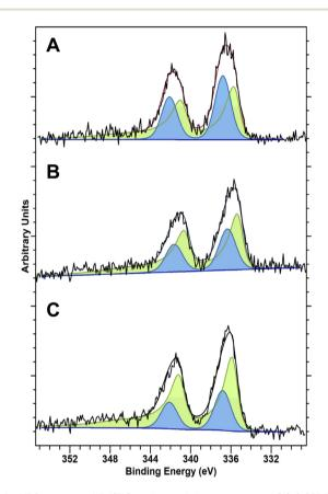
Fig. 1 XPS spectra of Pd(3d) regions of the as-prepared (A) 0.25%Pd-0.25%Sn/TiO<sub>2</sub>, (B) 0.25%Pd-0.25%Au/TiO<sub>2</sub> and (C) 0.5%Pd/TiO<sub>2</sub> catalysts. Key: Pd<sup>0</sup> (green) Pd<sup>2+</sup> (blue).
