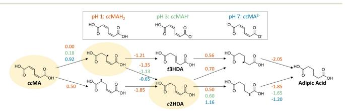
Fig. 1 Changes in free energy (eV) for the sequential addition of  $H^+|e^-$  pairs to cis,cis-muconic acid (ccMA) to form the hydrogenated hexenedioic acid and adipic acid products. Energetics are presented at -0.48 V vs. Ag/AqCl, the potential at which ccMA hydrogenation at pH 1 is calculated to have  $\Delta G = 0.00$  eV. The highlighted path shows the corresponding intermediates and products predicted by free energy calculations; t3HDA is formed experimentally.
