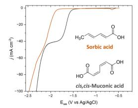
Fig. 5 Current–potential polarization curves on Pb RDE for 5 g  $L^{-1}$  solutions of sorbic acid and *cis,cis*-muconic acid at pH 7. The onset potential for the hydrogenation reaction shifted by 0.35 mV, from -1.55 V for *cis,cis*-muconic acid to -1.90 V for sorbic acid.
