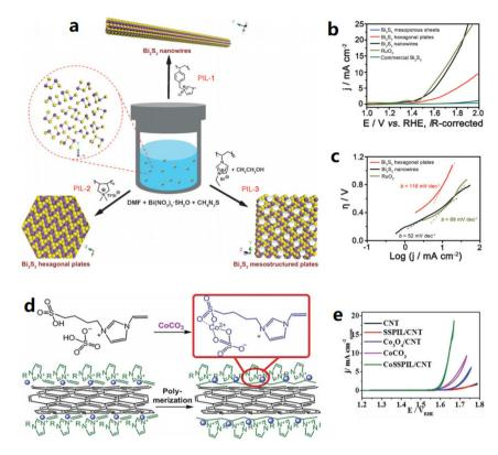
**Fig. 2** (a) PILs controlled the structures of  $Bi_2S_3$ , (b) OER linear sweep voltammetry (LSV) curves of  $Bi_2S_3$  and  $RuO_2$ , (c) Tafel slope of  $Bi_2S_3$  and  $RuO_2$ . Reproduced with permission.<sup>43</sup> Copyright 2016, Wiley-VCH; (d) preparation procedure of CoSSPIL/CNT, and (e) cyclic voltammogram (CV) of CoSSPIL/CNT compared to different samples of CNT, SSPIL/CNT,  $Co_3O_4/CNT$ , and  $CoCO_3$ . Reproduced with permission.<sup>44</sup> Copyright 2018, Wiley-VCH.
