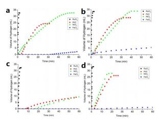
**Fig. 7** Metal-catalyzed hydrolytic H<sub>2</sub> release from the aqueous solution of (a)  $[Bu_4N][BH_3(NH_2BH_2)_2H]$ , (b)  $[Et_4N][BH_3(NH_2BH_2)_2H]$ , (c) [C  $(N_3H_6)][BH_3(NH_2BH_2)_2H]$ , and (d)  $[C(N_3H_5CH_3)][BH_3(NH_2BH_2)_2H]$  at room temperature.<sup>63</sup> Copyright 2021, Wiley-VCH.
