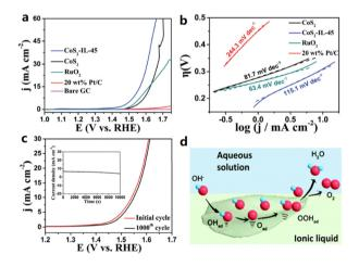
**Fig. 3** (a) OER LSV curves of the bare GC electrode, commercial 20 wt% Pt/C,  $CoS_2$  and IL-modified  $CoS_2$  and (b) the derived Tafel plots. (c) OER LSV curves of IL-modified  $CoS_2$  before and after 1000 CV tests. (d) Schematic illustration of the oxidation of water. Reproduced with permission.<sup>46</sup> Copyright 2018, the Royal Society of Chemistry.
