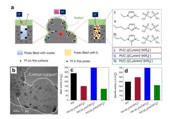
**Fig. 11** (a) The scheme of the ILs filled in the pores of carbon black supports. (b) The TEM images of Pt/C-IL catalysts. The gravimetric performance (c) and geometric performance (d) comparisons of catalysts modified with different ILs. Reproduced with permission from ref. 86. Copyright 2022, Springer Nature.
