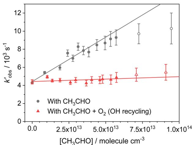
Fig. 6 Bimolecular plot of  $k'_{\text{obs}}$  vs. [CH<sub>3</sub>CHO] for the reaction between OH + CH<sub>3</sub>CHO (R5). Grey circles; OH loss with only CH<sub>3</sub>CHO present. Red triangles; OH loss with both CH<sub>3</sub>CHO and O<sub>2</sub> present. Curvature of the grey circles at [CH<sub>3</sub>CHO] above  $7 \times 10^{13}$  molecules per cm<sup>3</sup> indicates significant dimer formation, with the linear fits obtained only using data points below this.
