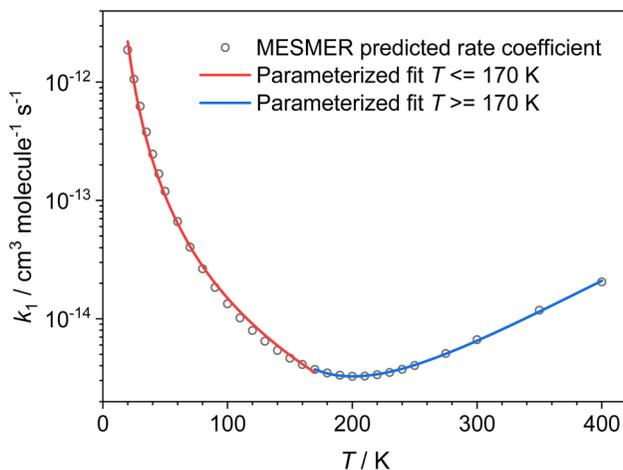
Fig. 8 Low-pressure limiting rate coefficients for the reaction between  $\text{NH}_2 + \text{CH}_3\text{CHO} \rightarrow \text{NH}_3 + \text{CH}_3\text{CO}$  (R1a) calculated by MESMER, using the PRC and TS energies determined by fitting to the experimental data (see text for details).
