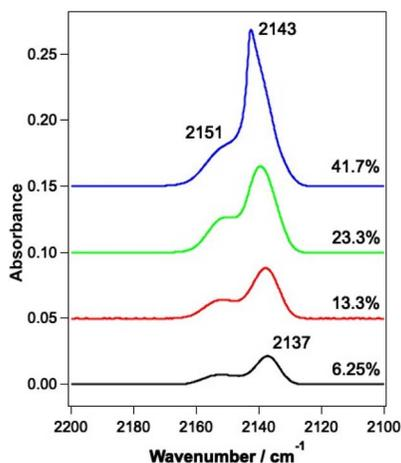
Fig. 2 RAIR spectra of mixtures of CO and water ranging from 6.25–41.7% CO with respect to 780  $L_m$  ASW. Ices were grown on the Au-plated Cu substrate at 18 K. Traces are offset vertically for clarity of presentation.
