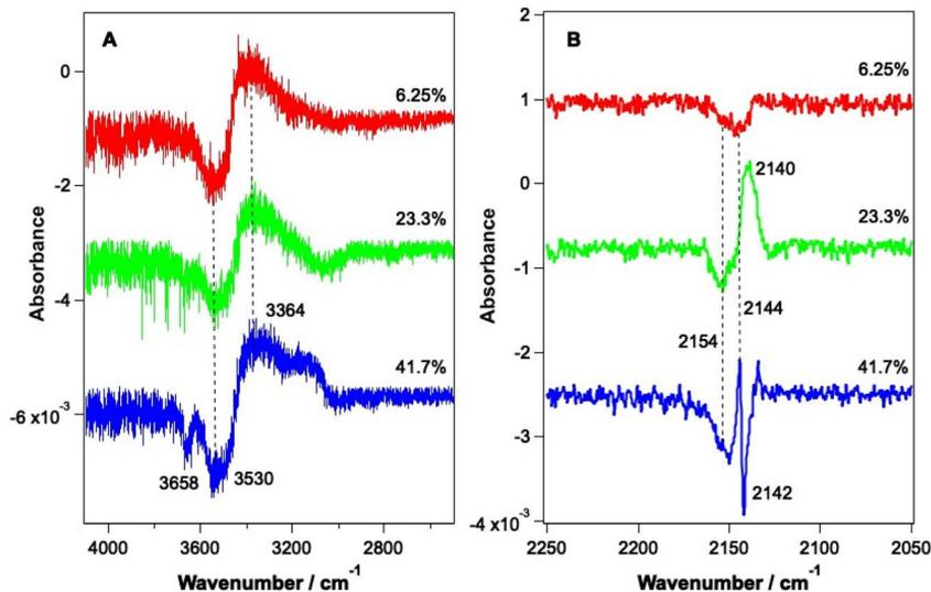
Fig. 5 RAIR difference spectra following the irradiation of various mixed ices at 2.9  $\mu\text{m}$  for 5 minutes. Irradiation energies were 1.6, 4 and 5 mJ for ices with compositions of 6.25%, 23.3% and 41.7%, respectively. (A) shows the O–H stretching region and (B) shows the C–O stretching region. Ice mixtures were dosed on Au-coated Cu at 18 K. Traces are offset vertically for clarity of presentation.
