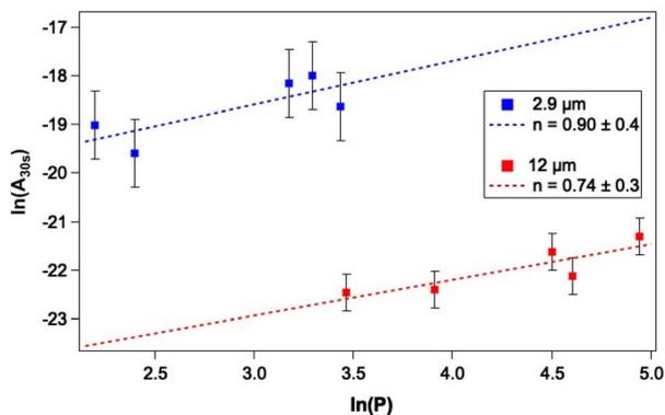
Fig. 9 Plot of  $\ln(A_{30s})$  as a function of  $\ln(P)$  to determine the laser power dependence of irradiation of mixed CO–water ices, comprising 13.3% CO with respect to 780  $L_m$  water ice dosed on Au-coated Cu at 18 K, at 2.9  $\mu\text{m}$  and 12  $\mu\text{m}$  for 5 minutes. Within the errors, excitation at both wavelengths is consistent with a single-photon process.
