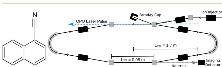
Fig. 1 (Left) Structure of 1-cyanonaphthalene (C<sub>10</sub>H<sub>7</sub>CN, 1-CNN). (Right) Schematic of DESIREE storage ring.
