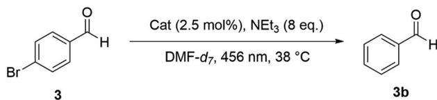
Scheme 2 Photocatalytic dehalogenation of 4-bromobenzaldehyde **3**.Table 1 Results of dehalogenation of **3** with different catalysts<sup>a</sup>
