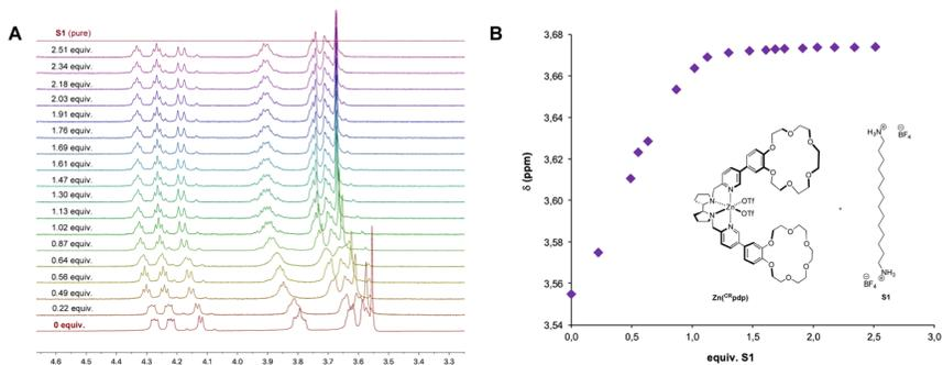
Fig. 2 Binding of **S1** to  $\text{Zn}^{\text{CR}}\text{pdp}$  (1 mM) in  $\text{CD}_3\text{CN}$  at 25 °C. (A) Enlargement of the region between 3.3 and 4.6 ppm, corresponding to the crown ether signals. (B) Titration curve.
