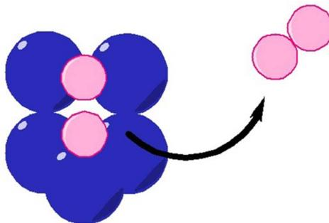
Fig. 1 Associative desorption of nitrogen (pink) at a Ru (blue)  $B_5$  active site: (1) nitrogen adatoms migrate to the  $B_5$  active site; (2) nitrogen adatoms associate to form molecular  $N_2$ ; (3) molecular  $N_2$  desorbs from  $B_5$  active site.
