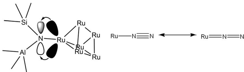
Fig. 17 Schematic (left) of Ru 5d to substituted N 2p back-donation with a  $\text{Ru}_6\text{N}_6$  cluster anchored to a bridging N to give electron deficient Ru atoms (only one Ru–N bond pictured, for clarity). Schematic (right) of decreasing Ru–N double bond character due to the electron deficient Ru atoms before the final desorption of Ru-bound molecular  $\text{N}_2$  during ammonia decomposition.
