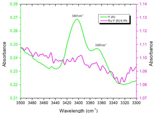
Fig. 4 FTIR spectra comparing the N–H stretching regimes of Y (N) and Ru–Y (N) 6.4%, collected at 400 °C in N<sub>2</sub> flow.
