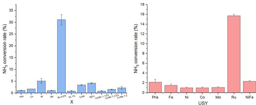
Fig. 14  $\text{NH}_3$  conversion rates of monometallic and bimetallic catalysts supported on X and USY at reaction conditions of 450 °C and 30 000 WHSV with pure ammonia feed gas. All metals were loaded in a M : Al ratio of 1 : 1, including each component of bimetallic catalysts, unless its wt% loading is given instead. Ratios for CoMo catalysts reflect Co : Mo ratio.
