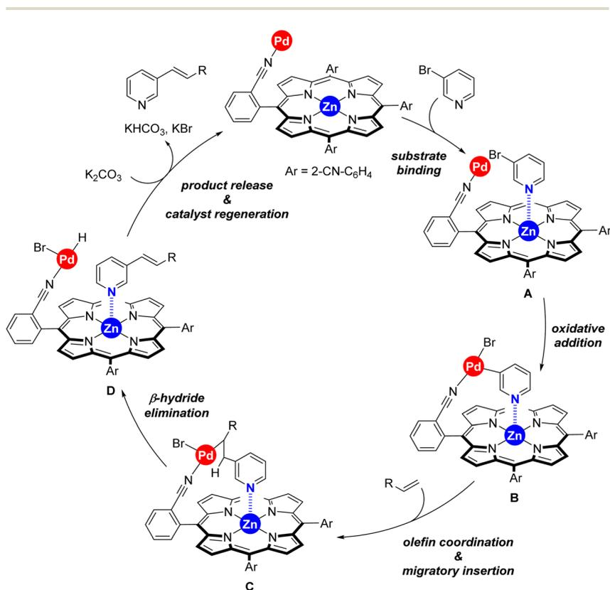
**Scheme 4** Postulated reaction mechanism for the supramolecular palladium-catalyzed Mizoroki–Heck cross-coupling reaction between 3-bromopyridine and terminal olefins exploiting remote, kinetically labile Zn $\cdots$ N weak interactions between the catalyst and the substrate.
