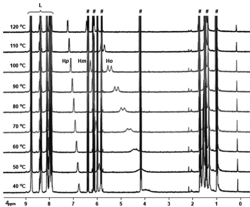
Fig. 2 Variable temperature  $^1\text{H}$  NMR (1,1,2,2-tetrachloroethane- $d_2$ , 400 MHz) spectra for the combination of L with 1 in the presence of excess 2a (for proton numbering see Scheme 1, # marks denote the proton signals belonging to the acrylate derivative 2a and L are the proton signals belonging to the supramolecular ligand L, and for concentration details see the ESI†).
