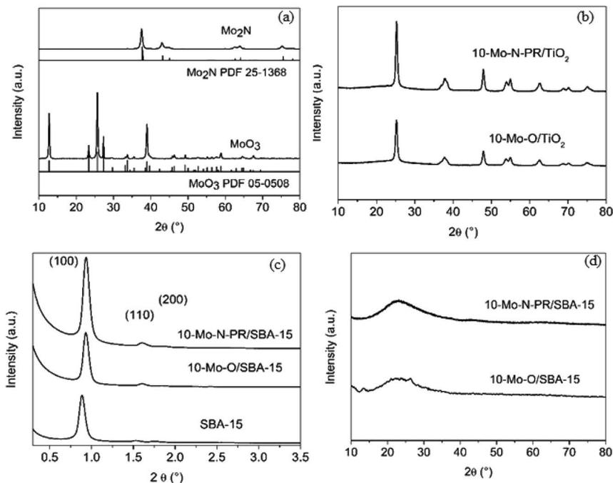
Fig. 1 XRD diffractograms of (a) unsupported  $\alpha\text{-MoO}_3$  and  $\beta\text{-Mo}_2\text{N}$ , (b) 10-Mo-O/TiO<sub>2</sub> and 10-Mo-N-PR/TiO<sub>2</sub>, (c) SAXS diffractograms of 10-Mo-O/SBA-15 and 10-Mo-N-PR/SBA-15 and (d) wide angle domain diffractograms of 10-Mo-O/SBA-15 and 10-Mo-N-PR/SBA-15. \*10-Mo-N-PR/TiO<sub>2</sub> and 10-Mo-N-PR/SBA-15 are post-ammonia synthesis reaction catalysts obtained after 1000 min in stream.
