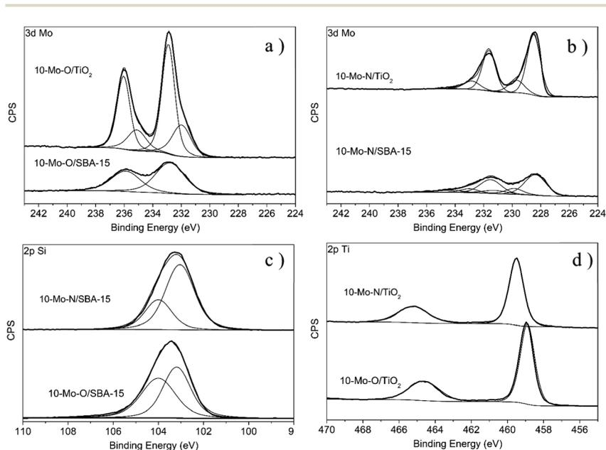
Fig. 4 XPS spectra recorded for the calcined materials (10-Mo-O/SBA-15 and 10-Mo-O/TiO<sub>2</sub>) and after nitridation under reaction conditions at 700 °C for 2 h in the environmental XPS chamber. (a) Mo 3d region: 10-Mo-O/SBA-15 and 10-Mo-O/TiO<sub>2</sub>, (b) Mo 3d region: 10-Mo-N/TiO<sub>2</sub> and 10-Mo-N/SBA-15, (c) Si 2p region: 10-Mo-O/SBA-15 and 10-Mo-N/SBA-15 and (d) Ti 2p region: 10-Mo-O/TiO<sub>2</sub> and 10-Mo-N/TiO<sub>2</sub>.
