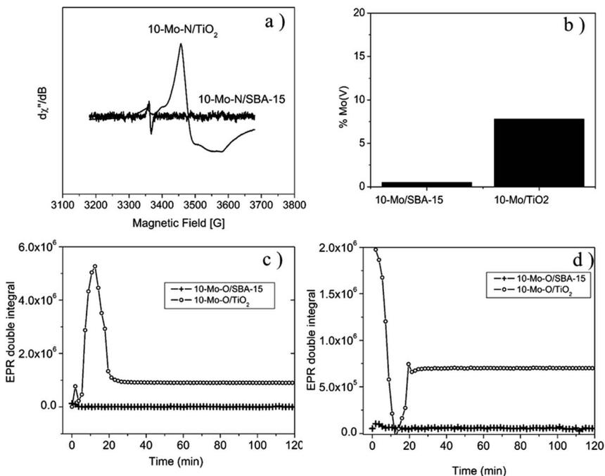
Fig. 5 EPR results: (a) EPR spectra after reaction, (b) fraction of  $\text{Mo}^{5+}$  after pre-treatment, (c) kinetic evolution of  $\text{Mo}^{5+}$  species at  $700\text{ }^\circ\text{C}$  under hydrogen, and (d) kinetic evolution of  $\text{O}^{1-}$  species at  $700\text{ }^\circ\text{C}$  under  $\text{H}_2/\text{N}_2$ .
