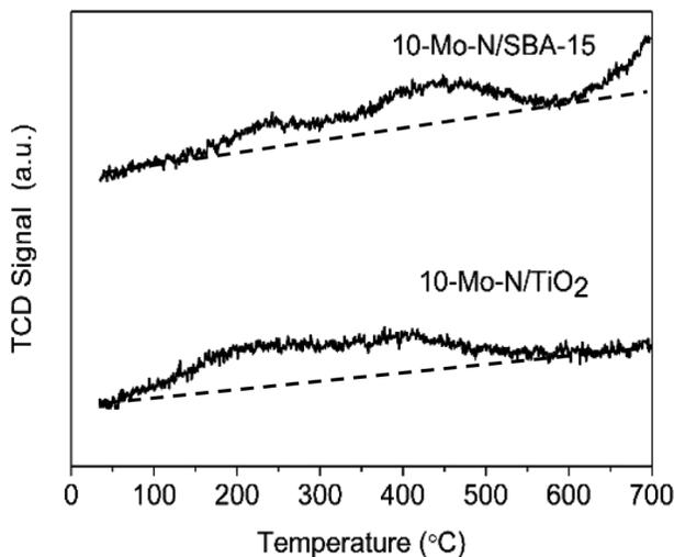
Fig. 7  $\text{H}_2$ -TPD profiles of 10-Mo-N/SBA15 and 10-Mo-N/TiO<sub>2</sub>.
