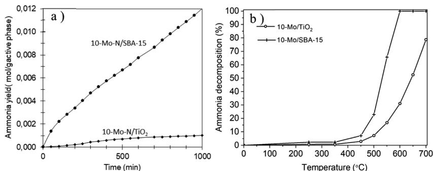
Fig. 8 (a) Cumulative ammonia yield obtained for 10-Mo-N/SBA-15 and 10-Mo-N/TiO<sub>2</sub>. Reaction performed under 60 mL min<sup>-1</sup> flow rate of 75 vol% H<sub>2</sub>/N<sub>2</sub> at 400 °C and ambient pressure. (b) Ammonia decomposition conducted under 15% NH<sub>3</sub> in Ar at different temperatures and atmospheric pressure.
