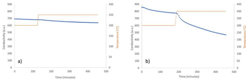
Fig. 9 Ammonia production reaction profiles of  $\text{Ni}_3\text{CuN}$  reacted with  $60 \text{ mL min}^{-1}$  of 3 : 1  $\text{H}_2/\text{N}_2$  (a) for 2 hours 5 minutes at  $200 \text{ }^\circ\text{C}$  and 5 hours 25 minutes at  $250 \text{ }^\circ\text{C}$  and (b) for 3 hours at  $300 \text{ }^\circ\text{C}$  and 4 hours 25 minutes at  $400 \text{ }^\circ\text{C}$ .
