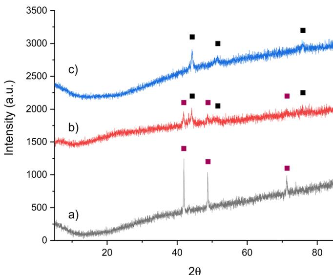
Fig. 1 XRD patterns of Co<sub>3</sub>CuN: (a) pre-reaction, (b) post-reaction with 3 : 1 H<sub>2</sub>/N<sub>2</sub> at 200 °C and 250 °C and (c) post-reaction with 3 : 1 H<sub>2</sub>/N<sub>2</sub> at 300 °C and 400 °C. (■) Co<sub>3</sub>CuN and (■) Co<sub>3</sub>Cu.
