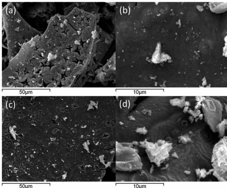
Fig. 17 Representative SEM images of 'Co<sub>3</sub>MoN': (a and b) pre-reaction and (c and d) post N<sub>2</sub>/H<sub>2</sub> reaction at 400 °C.
