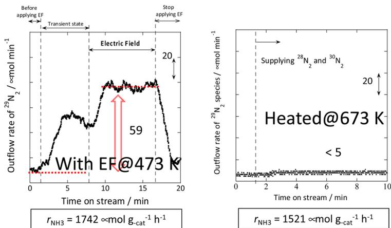
Fig. 7 Isotope exchange tests using  $^{30}\text{N}_2$ : (left) with the electric field at 473 K and (right) without the electric field at 673 K. Catalyst, 9.9 wt% Cs/5.0 wt% Ru/SrZrO<sub>3</sub>, 200 mg; flow,  $^{28}\text{N}_2$  :  $^{30}\text{N}_2$  : H<sub>2</sub> : Ar = 6 : 6 : 36 : 12 SCCM; either 0 or 6 mA current.<sup>30</sup>
