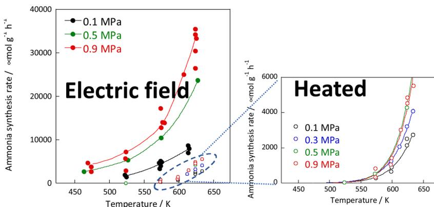
Fig. 2 Reaction rates of ammonia synthesis over 9.9 wt% Cs/5.0 wt% Ru/SrZrO<sub>3</sub> catalyst with and without the electric field: 200 mg catalyst, 0 or 6 mA current, H<sub>2</sub> : N<sub>2</sub> = 3 : 1, 240 SCCM total flow rate.
