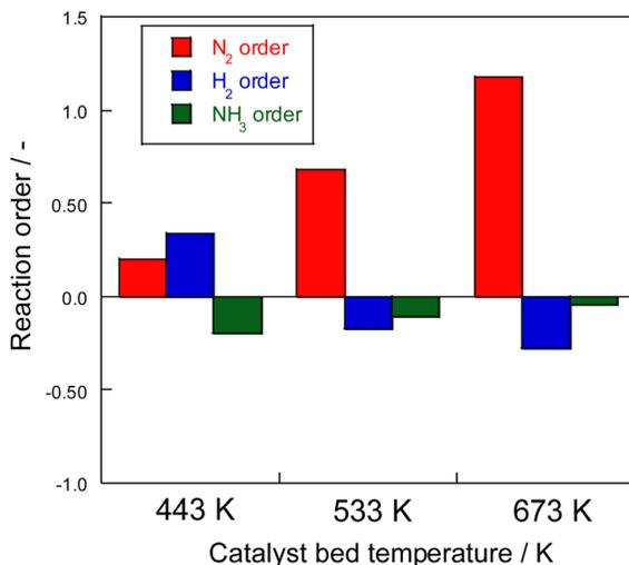
Fig. 5 Reaction order of ammonia synthesis over 1 wt% Ru/CeO<sub>2</sub> catalyst with the electric field: 100 mg catalyst, 0 or 6 mA current, 240 SCCM total flow rate.
