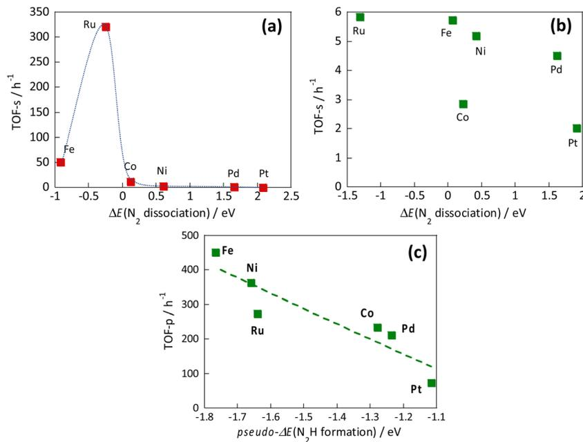
Fig. 13 Correlation between the  $N_2$  dissociation energy and the TOF-s of the catalytic reaction upon heating (a), correlation when the electric field is applied (b), and correlation between  $N_2\text{H}$  formation energy and TOF-p (c).<sup>36</sup>
