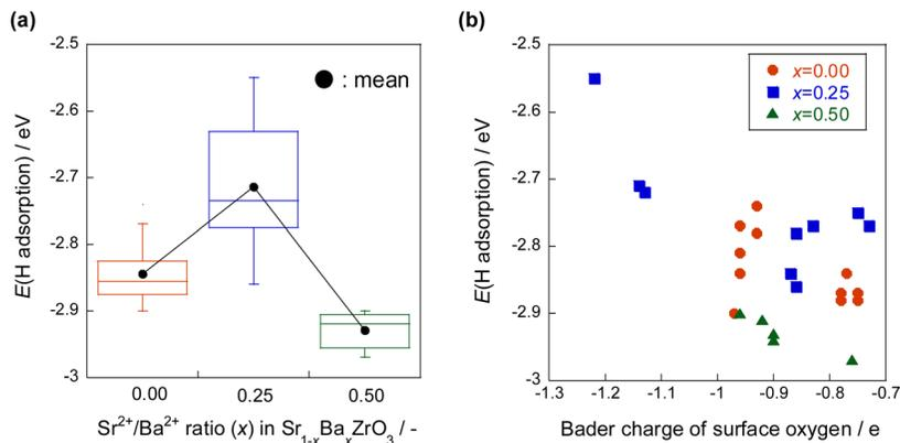
Fig. 15 Hydrogen atom adsorption energies for  $\text{Sr}_{1-x}\text{Ba}_x\text{ZrO}_3$  ( $0 \leq x \leq 0.5$ ) by DFT calculations, (a) the effect of Sr/Ba ratio, (b) the effect of Bader charge of surface oxygen.<sup>44</sup>
