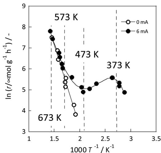
Fig. 3 Reaction rate of ammonia synthesis over 1 wt% Ru/CeO<sub>2</sub> catalyst with and without the electric field: 100 mg catalyst, 0 or 6 mA current, H<sub>2</sub> : N<sub>2</sub> = 3 : 1, 240 SCCM total flow rate.<sup>31</sup>
