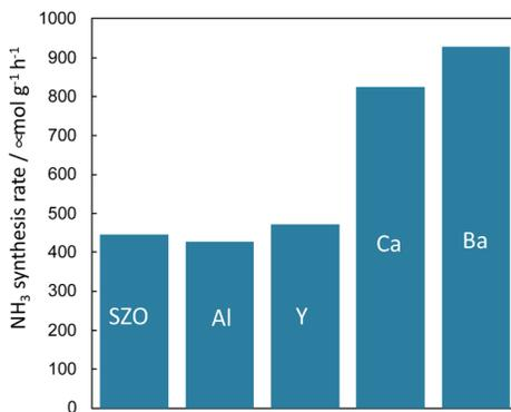
Fig. 11 Effects of different cation doping into SrZrO<sub>3</sub> support on the ammonia synthesis rate in the electric field using Ru as a supported metal: 100 mg catalyst, 6 mA current, H<sub>2</sub> : N<sub>2</sub> = 3 : 1, 240 SCCM total flow rate.<sup>38</sup>
