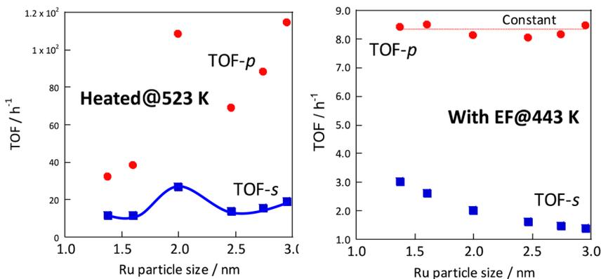
Fig. 4 Turnover frequency over Ru catalysts supported on CeO<sub>2</sub> having various Ru particle sizes with and without heating or an electric field: 0.5–5 wt% Ru, 100 mg catalyst, 0 or 6 mA current, H<sub>2</sub>: N<sub>2</sub> = 3 : 1, 240 SCCM total flow rate.
