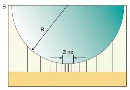
Fig. 1 (A) Simplified basic set-up for STM. Reproduced with permission. Copyright © 2021, Springer Nature Limited. (B) Estimation of the lateral resolution in STM. Reproduced with permission. Copyright © 1993, Oxford University Press.
