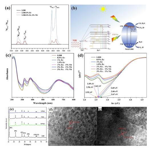
Fig. 12 (a) Upconversion emission spectra of LDH, LDH:1% Er, and LDH:1% Er,2% Yb, (b) schematic diagram of photocatalytic CO<sub>2</sub> reduction under the irradiation of UV-Vis and NIR light, (c) UV-Vis DRS, (d) band-gap energies of the as-prepared samples, (e) XRD patterns of different contents of Er<sup>3+</sup> doped LDH, (f and g) HRTEM images of pure LDH, LDH:1% Er (Figures taken with permission from ref. 147 copyright 2023, Elsevier).
