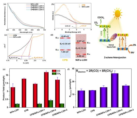
Fig. 23 (a) UV-Vis DRS spectra of NiFe-LDH and CPB/LDH-x (x = 1-3), (b and c) VB-XPS spectra and Tauc-plots of CPB and NiFe-LDH, (d) energy band alignments of CPB and NiFe-LDH, (e) the product yield rates of the photocatalysts, (f) the electron consumption of pristine NiFe-LDH, CPB and CPB/ NiFe-LDH-x (x = 1-3) (Figures taken with permission from ref. 111 copyright 2023, RSC).
