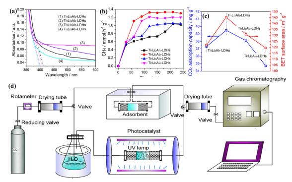
Fig. 6 UV-Vis DRS spectra of (a) Ti/Li/Al-LDHs with different Ti:Li:Al molar ratios. Photocatalytic CH<sub>4</sub> yields of (b) Ti/Li/Al-LDHs with different Ti:Li:Al molar ratios. Surface area and the adsorption capacity of CO<sub>2</sub> for (c) Ti/Li/Al-LDHs with different Ti: Li: Al molar ratios, (d) schematic of the apparatus for CO<sub>2</sub> adsorption and photocatalytic CO<sub>2</sub> reduction (Figures taken with permission from ref. 131 copyright 2023, Nature).
