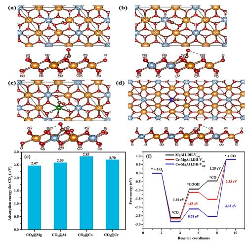
Fig. 14 Optimized structural models of CO<sub>2</sub> adsorption over (a) Mg, (b) Al, (c) Co and (d) Cr sites (Atoms in different colors: yellow-Mg, light blue-Al, green-Co, blue-Cr, red-O, white-H, black-C), (e) CO<sub>2</sub> adsorption energies over different metal sites, and (f) free energy diagram describing the COOH\* intermediate from CO<sub>2</sub> to CO over three LDHs (Figures taken with permission from ref. 149 copyright 2023, Elsevier).
