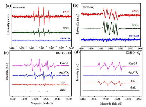
Fig. 21 The ESR spectrum of the type-II  $g-C_3N_4$  foam/LDH photocatalyst (a and b) and Z-Scheme  $g-C_3N_4/Ag_3VO_4/r$ -GO photocatalyst (c and d) (Figures taken with permission from ref. 182 and 117 copyright 2023, Elsevier).
