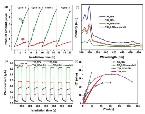
Fig. 18 (a) Recycling tests of  $CH_4$  and CO evolution over the  $TiO_2/LDH$  core-shell hybrid, (b) steady-state PL spectra, (c) photocurrent responses, and (d) EIS profiles of the  $TiO_2$  NPs,  $TiO_2$  HSs,  $TiO_2$  NPs/LDH, and  $TiO_2/LDH$  core-shell hybrid sample (Figures taken with permission from ref. 174 copyright 2023, RSC).
