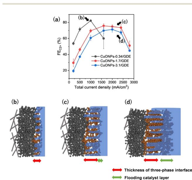
Fig. 4 (a) FE<sub>C<sub>2+</sub></sub> against  $J_{total}$  for various amounts of Cu loading (CuONPs-0.34, -1.7 and -3.1/GDE) in 1 M KCl. (b–d) Schematic image of the three-phase interfaces at each position which are indicated in (a). The red and green arrows represent the thickness of three-phase interface and flooding catalyst layer, respectively.
