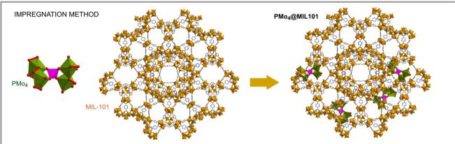
Scheme 2 Representation of the two distinct experimental procedures applied for the preparation of the composite materials: one-pot method (used for the preparation of PMo<sub>4</sub>@MOF-808, top, and PMo<sub>4</sub>@ZIF-8) and the impregnation method (used to prepare PMo<sub>4</sub>@MIL-101, bottom).
