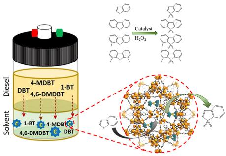
Scheme 3 Illustration of the ECODS processes using heterogeneous PMo<sub>4</sub>@MOFs catalysts.
