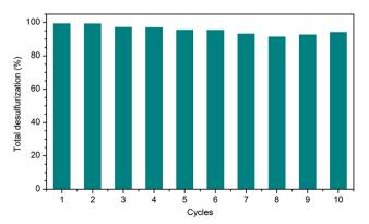
Fig. 6 Reusability of the homogeneous PMo<sub>4</sub> (7.5 μmol) catalyst using 0.75 mL of [BMIM]PF<sub>6</sub> extraction solvent, 0.78 mmol of H<sub>2</sub>O<sub>2</sub>, and 7.5 μmol of PMo<sub>4</sub> at 70 °C. The results were obtained at 2 h.
