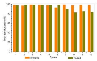
Fig. 8 Recyclability and reusability of ECODS system using the PMo<sub>4</sub>@MIL-101 catalyst under the optimized conditions (catalyst containing 7.5 µmol of PMo<sub>4</sub>, 0.75 mL of extraction solvent [BMIM]PF<sub>6</sub>, and 0.78 mmol of H<sub>2</sub>O<sub>2</sub> at 70 °C). Results were obtained after 2 h.
