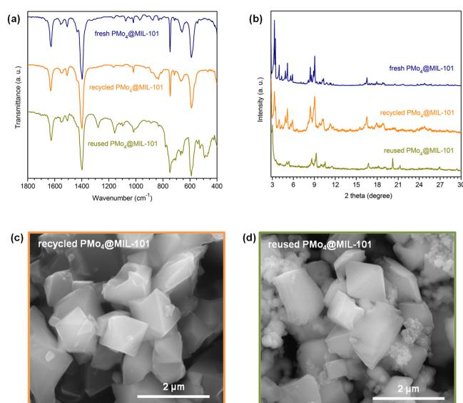
Fig. 9 Characterization data obtained for fresh, recycled, and reused PMo₄@MIL-101 heterogeneous catalysts: FT-IR spectra (a), powder XRD patterns (b), and SEM images (c and d).
