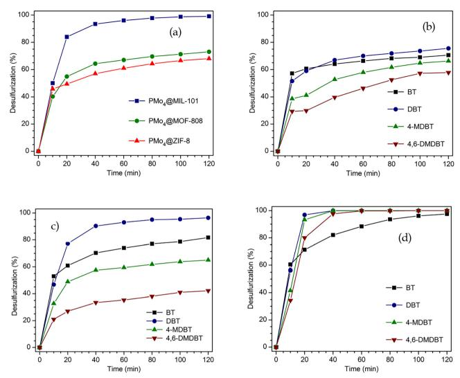
Fig. 7 Desulfurization profile of the multicomponent model diesel (2000 ppm of S) catalyzed by PMo<sub>4</sub>@MOFs, containing 7.5 μmol PMo<sub>4</sub> with 0.75 mL of [BMIM]PF<sub>6</sub> as the extraction solvent and 0.78 mmol H<sub>2</sub>O<sub>2</sub> at 70 °C (a). Desulfurization profile of each sulfur compound present in the model diesel catalyzed by PMo<sub>4</sub>@ZIF-8 (b), PMo<sub>4</sub>@MOF-808 (c), and PMo<sub>4</sub>@MIL-101 (d).
