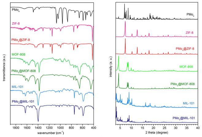
Fig. 1 FT-IR spectra showed in the wavenumber range 1900–400 cm $^{-1}$  (left-hand side) and powder XRD patterns showed between 2 and 40 $^{\circ}$  (right-hand side) from PMo $_4$ , pristine MOFs, and PMo $_4$ @MOFs composites.
