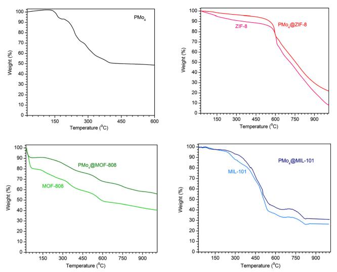
Fig. 3 TGA curves for PMo₄ (top left), ZIF-8 and PMo₄@ZIF-8 (top right), MOF-808 and PMo₄@MOF-808 (bottom left), MIL-101(Cr) and PMo<sub>4</sub>@MIL-101(Cr) (bottom right).
