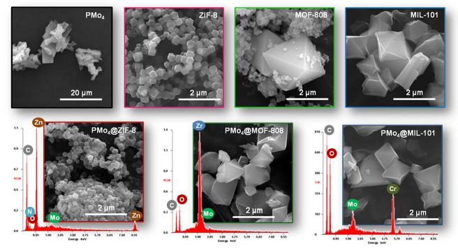
Fig. 2 SEM images of PMo<sub>4</sub>, the pristine MOFs (ZIF-8, MOF-808, and MIL-101), and the composites (PMo<sub>4</sub>@ZIF-8, PMo<sub>4</sub>@MOF-808, and PMo<sub>4</sub>@MIL-101) overlaid by the corresponding EDX spectra.
