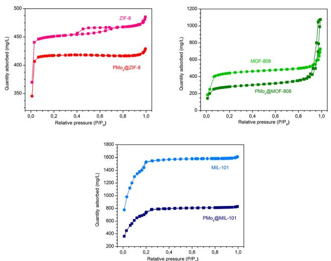
Nitrogen adsorption-desorption isotherms at −196 °C for MOFs and the corresponding PMo<sub>4</sub>@MOFs composites.
