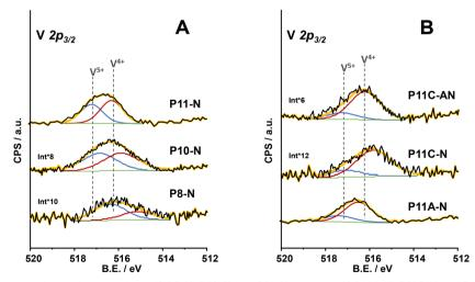
Fig. 5 XPS results of V 2p<sub>3/2</sub> core level of the catalysts: A) P8-N; P10-N and P11-N catalysts; B) P11A-N; P11C-N and P11C-aN catalysts.
