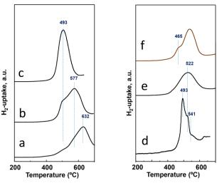
Fig. 4 H<sub>2</sub>-uptake during the TPR-H<sub>2</sub> experiments for activated catalysts: a) P8-N; b) P10-N; c) P11-N; d) P11A-N; e) P11B-N; f) P11CaN. Characteristics of the catalysts are shown in Table 1.
