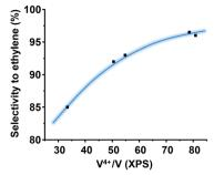
Fig. 8 Variation of the selectivity to ethylene during the ethane ODH with the V<sup>4+</sup> content on the catalyst surface, determined by XPS. Reaction conditions for ethane ODH: 25% ethane conversion and a reaction temperature of 412 °C, and remaining conditions in the text.
