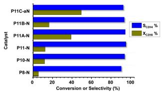
Fig. 7 Variation of ethane conversion  $(X_{C_2H_{\epsilon'}}, \%)$  and selectivity to ethylene (S<sub>C,H,</sub>, %) during the ethane ODH over MoVTeNbO catalysts at a reaction temperature of 400 °C. Experimental conditions in the
