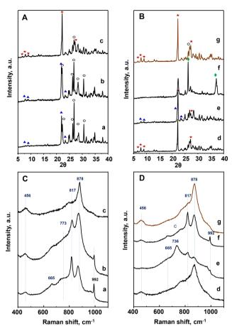
Fig. 1 XRD patterns (A and B) and Raman spectra (C and D) of heattreated catalysts: a) P8-N; b) P10-N; c) P11-N; d) P11A-N; e) P11B-N; f) P11C-N; g) P11C-aN. Characteristics of the catalysts are shown in Table 1. Symbols: M1 phase (\*);  $TeMo_5O_{16}$  ( $\circ$ );  $Mo_5O_{14}$  ( $\triangle$ );  $MoO_2$  ( $\diamondsuit$ ).
