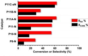
Fig. 6 Variation of propane conversion ( $X_{C_2H_0}$ , %) and selectivity to acrylic acid ( $S_{AA}$ , %) during partial oxidation of propane over MoVTeNbO catalysts at a reaction temperature of 380 °C. Experimental conditions in the text.
