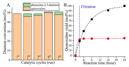
Fig. 3 Five run recycling test (A) and the hot filtration test (B) of the CoBi<sub>2</sub>O<sub>2</sub>CO<sub>3</sub> catalyst. Reaction conditions: 1 equiv. (0.25 M) o-phenylenediamine, 2 mL ethylene glycol, 110 °C for 24 h (4 h in the case of recycling) and 2.5 mol% catalyst.
