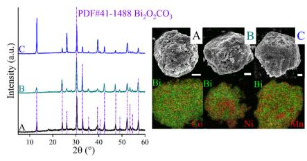
Fig. 1 XRD patterns, SEM images and SEM-EDX elemental maps of CoBi<sub>2</sub>O<sub>2</sub>CO<sub>3</sub> (A); NiBi<sub>2</sub>O<sub>2</sub>CO<sub>3</sub> (B) and MnBi<sub>2</sub>O<sub>2</sub>CO<sub>3</sub> (C). The scale bars represent 400 nm. The purple dashed-dot lines represent the positions and intensities of the characteristic reflections of a pure bismuth subcarbonate sample (bismutite, Bi<sub>2</sub>O<sub>2</sub>CO<sub>3</sub>).
