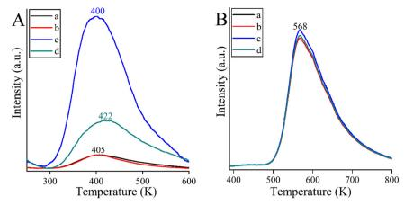
Fig. 4 CO<sub>2</sub>-TPD curves (A) and NH<sub>3</sub>-TPD curves (B) of the bismutite-based composites: Bi<sub>2</sub>O<sub>2</sub>CO<sub>3</sub> (a), MnBi<sub>2</sub>O<sub>2</sub>CO<sub>3</sub> (b), COBi<sub>2</sub>O<sub>2</sub>CO<sub>3</sub> (c) and NiBi<sub>2</sub>- $O_2CO_3$  (d).
