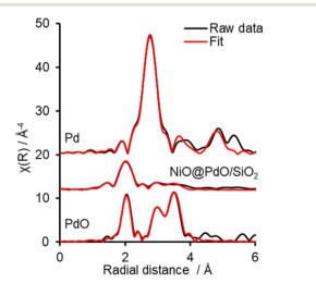
Fig. 2 EXAFS Fourier transforms and fits for PdO and Pd references and NiO@PdO/SiO2.
