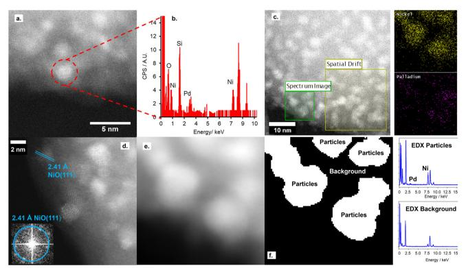
Fig. 1 a. High-angle annular dark field (HAADF)-STEM of NiO@PdO/SiO2, b. selected area energy dispersive X-ray (EDX) spectrum of highlighted nanoparticles, c. EDX mapping of NiO@PdO/SiO2, d. atomic resolution imaging of NiO@PdO/SiO2 with Fourier transform of the STEM image (inset), and e. and f. HAADF-STEM imaging and applied particle and background mask for EDX spectra subtractions with corresponding EDX spectra.
