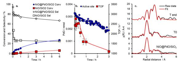
Fig. 3 a. Selox reaction and selectivity profiles for NiO@PdO/SiO<sub>2</sub> and NiO/SiO<sub>2</sub>, b. evolution of catalytic PdO content and instantaneous TOFs derived from LCF of *operando* Pd K edge XAS during cinnamyl alcohol selox, and c. FT EXAFS and fit of *ex situ* and *operando* NiO@PdO/SiO<sub>2</sub> at T<sub>0</sub> and 6 hours.
