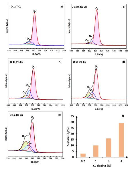
Fig. 5 X-ray photoelectron spectra of O 1s: a) TiO2, b) 0.2% Cu/TiO2, c) 1% Cu/TiO2, d) 3% Cu/TiO2 and e) 4% Cu/TiO2. f) Correlation between surface O<sub>V</sub> (normalized area in XPS) and doping concentration.
