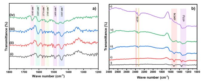
Fig. 6 a) Pyridine DRIFTS spectra of Cu/TiO2 at (i) 323 K, (ii) 373 K, (iii) 473 K and (iv) 573 K. b) DRIFTS measurements during oxidation of ethylene using 1% Cu/TiO<sub>2</sub> with a mixture of ethylene (1.5 vol%) and oxygen (5.9 vol%) at (i) 298 K; (ii) 373 K; (iii) 473 K; (iv) 573 K; (v) 673 K.
