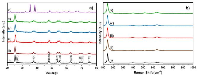
Fig. 1 a) XRD patterns of i) TiO<sub>2</sub> (black), ii) 0.2% Cu/TiO<sub>2</sub> (brown), iii) 1% Cu/TiO<sub>2</sub> (red), iv) 3% Cu/TiO<sub>2</sub> (blue), v) 4% Cu/TiO<sub>2</sub> (green) and vi) bulk CuO (violet). b) Raman spectra of i) TiO<sub>2</sub> (black), ii) 0.2% Cu/TiO<sub>2</sub> (brown), iii) 1% Cu/TiO<sub>2</sub> (red), iv) 3% Cu/TiO<sub>2</sub> (blue) and v) 4% Cu/TiO<sub>2</sub> (green).
