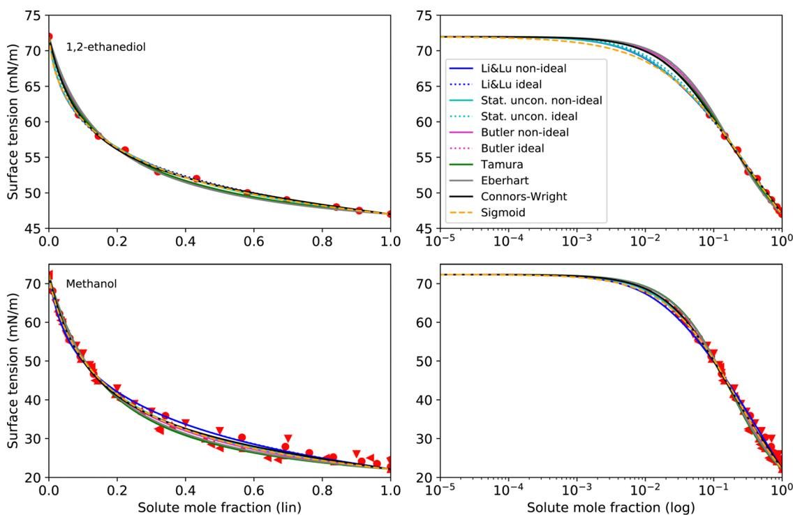
**Fig. 3** Surface tension fits (lines) and experimental data (red symbols) for 1,2-ethanediol and methanol on linear (left) and logarithmic scales (right). Different symbols of the experimental data refer to different sources (see Table 2 and Fig. S2 in ESI†).
