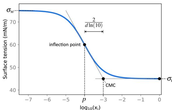
Fig. 2 Illustration of the Sigmoid model (blue solid line, eqn (25)) with parameters  $\sigma_w = 75 \text{ mN m}^{-1}$ ,  $\sigma_i = 45 \text{ mN m}^{-1}$ ,  $p = -4$ , and  $d = 0.869$ . The critical micelle concentration ‘‘CMC’’ is estimated by intersecting the tangent line at the inflection point with a horizontal line at  $\sigma(x_i \rightarrow \infty)$ .
