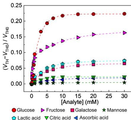
**Fig. 3** Response profiles of the GO-OFET-based chemical sensor with 4-MPBA against seven analytes in 0.1 M phosphate buffer with 0.1 M NaCl at pH 7.4. Titration isotherms were obtained by collecting  $V_{TH}$  at each concentration of analytes from 0 to 30 mM. The terms  $V_{TH0}$  and  $V_{TH}$ , respectively, indicate threshold voltages before and after adding the analytes. Three repetitive evaluations were carried out for each analyte.
