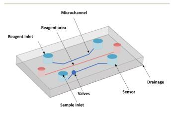
Fig. 3 The general structure of a microfluidic chip.
