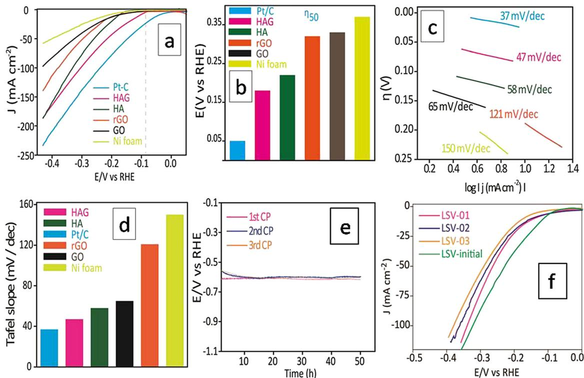
Fig. 7 HER electrocatalytic performance of HAG. (a) Polarograms of HAG, HA, rGO, GO, Pt-C, and Ni foam is taken at 2 mV s<sup>-1</sup> without iR correction. (b) Bar diagram showing the η<sub>50</sub> values of all materials. (c) Tafel slope comparison. (d) Bar diagram showing the Tafel slope values compared between the catalysts. (e) Chronoamperometric stability experiment and activity reproducibility test of HAG. (f) Polarograms recorded after each CP experiment.
