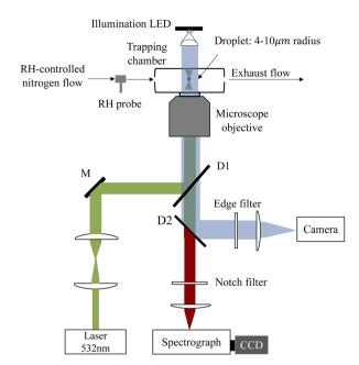
Fig. 1 Schematic of the aerosol optical tweezers system. A laser beam passes through a pair of beam expansion optics and finally couples into an objective to form the laser tweezers. The droplet is imaged using a 470 nm illumination LED and a high frame rate camera. The Raman spectra of the trapped droplets are recorded using a spectrograph/ CCD. M is a mirror. D1 and D2 are dichroic mirrors.
