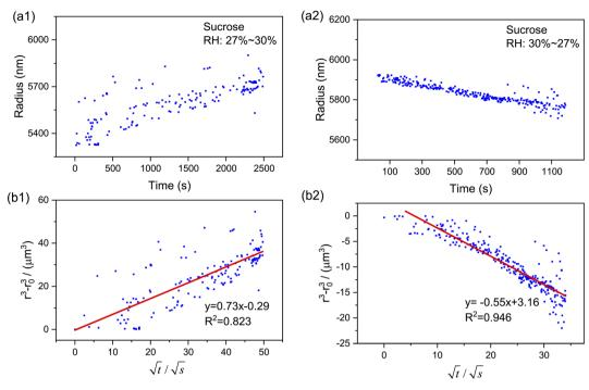
Fig. 4 Size-response of the sucrose droplets to RH changes. Time evolution of the radius when RH changed from 27% to 30% (a1) and from 30% to 27% (a2), respectively. Relationship of  $r^3 - {r_0}^3$  and  $\sqrt{t}$  when RH changed from 27% to 30% (b1) and from 30% to 27% (b2), respectively. Linear regressions are plotted in red lines.
