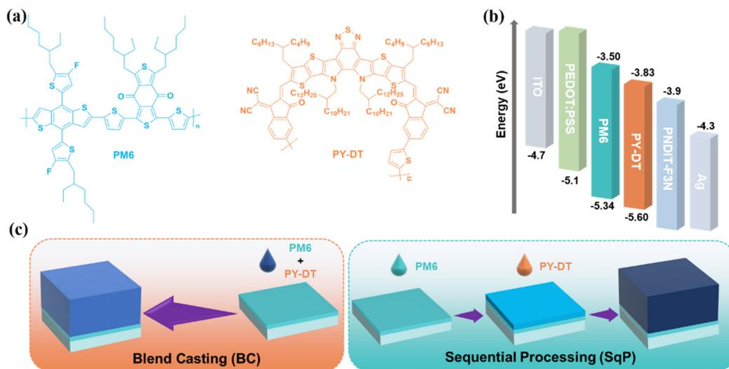
Fig. 1 (a) Chemical structures of polymer donor PM6 and polymer acceptor PY-DT. (b) Energy level distribution of materials in our devices. (c) Processing schematic diagram of BC and SqP methods.
