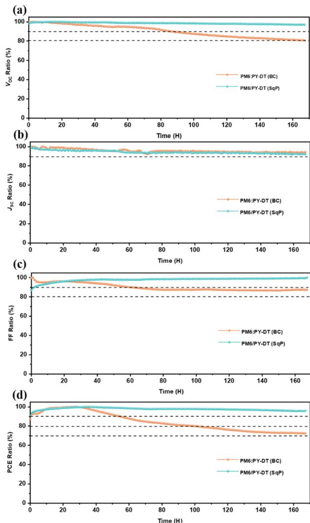
Fig. 6 MPP tracking results for BC and SqP devices: (a)  $V_{OC}$ , (b)  $J_{SC}$ , (c) FF and (d) PCE.
