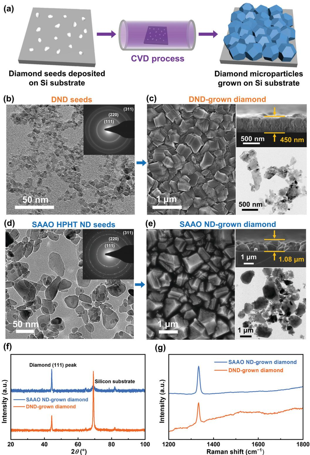
**Fig. 1** (a) Schematic illustration of the CVD process. (b) TEM (inset: SAED pattern) image of the DND seeds and (c) corresponding SEM, cross-section SEM and TEM images of the DND-grown diamond microparticles. (d) TEM (inset: SAED pattern) image of the SAAO HPHT ND seeds and (e) corresponding SEM, cross-section SEM and TEM images of the SAAO ND-grown diamond microparticles. (f) XRD and (g) Raman spectra of the CVD-grown diamond microparticles.
