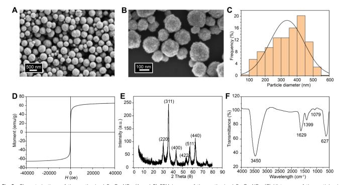
Fig. 2 Characterizations of the synthesized Fe<sub>3</sub>O<sub>4</sub> NPs. (A and B) SEM images of the synthesized Fe<sub>3</sub>O<sub>4</sub> NPs. (C) Histogram of the particle size distribution. (D) The magnetization curves of Fe<sub>3</sub>O<sub>4</sub> particles at 37 °C. Inset: Close-up of the hysteresis at H = 0. (E) The XRD pattern of the synthesized Fe<sub>3</sub>O<sub>4</sub> NPs. (F) The FTIR spectrum of the synthesized Fe<sub>3</sub>O<sub>4</sub> NPs.
