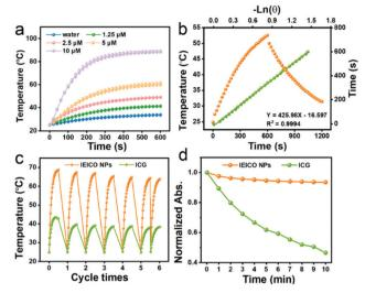
Fig. 2 (a) Time-dependent temperature variation of IEICO NP aqueous solutions with different concentrations under 808 nm laser irradiation (1 W cm $^{-2}$ ). (b) Photothermal conversion efficiency of IEICO NPs. (c) The temperature changes of IEICO NPs (10  $\mu$ M) and ICG (10  $\mu$ M) in aqueous solutions under 808 nm laser for 6 cycles. (d) Time-dependent normalized absorbance of IEICO NPs and ICG.
