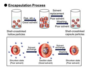
Scheme 2 Schematic illustration of solvent exchange procedures applied to P(CEA-CEMA)-50 particles for the preparation of capsule particles. P(CEA-CEMA): poly(2-carboxyethylacrylate-co-2-cinnamoylethyl methacrylate)
