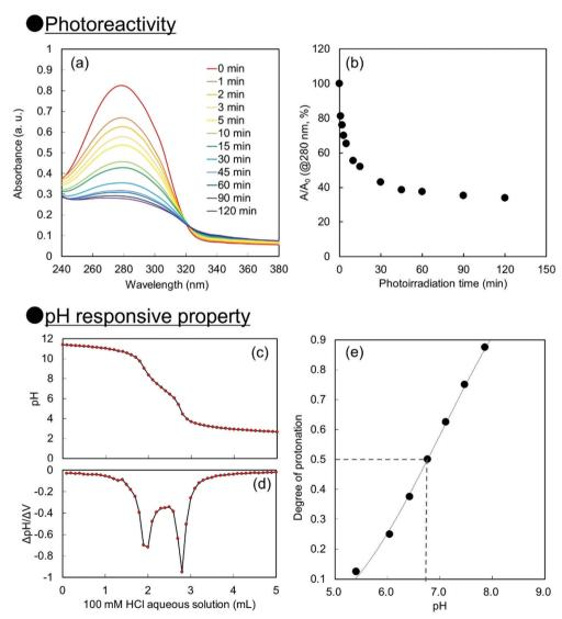
Fig. 1 (a) UV-Vis spectra and (b) absorbance changes at  $\lambda$  = 280 nm of P(CEA-CEMA)-50 thin film prepared on a quartz substrate after various photoirradiation periods. (c) pH titration curve, (d) differential of the pH curve, and (e) degree of protonation under various pH conditions of P(CEA-CEMA)-50 in water. P(CEA-CEMA): poly(2-carboxyethylacrylate-co-2-cinnamoylethyl methacrylate).
