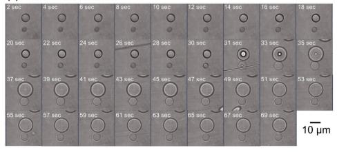
Fig. 3 Time lapse images of NaOH added aqueous dispersion of P(CEA-CEMA)-50 particles (a) before and (b) after interfacial photocrosslinking. P(CEA-CEMA): poly(2-carboxyethylacrylate-co-2-cinnamoylethyl methacrylate).
