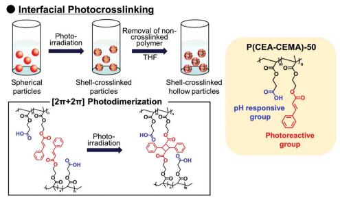
Scheme 1 Schematic illustration of interfacial photocrosslinking of P(CEA-CEMA)-50 particles for the preparation of hollow particles. pH-responsive release of P(CEA-CEMA)-50 capsule particles. P(CEA-CEMA): poly(2-carboxyethylacrylate-co-2-cinnamoylethyl methacrylate).
