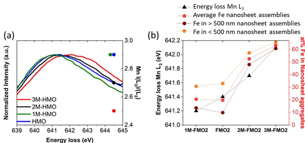
Fig. 8 (a) Left-Y Axis: EELS Mn  $L_3$  peaks of HMO, 1M-HMO, 2M-HMO and 3M-HMO. Right-Y axis: corresponding Mn  $L_3/L_2$  values. (b) Trends of oxidation state of  $x\text{M-HMO}$  (Left-Y axis) and Fe introduced by galvanic exchange reaction (right-Y axis) for  $x\text{M-FMO2}$ .
