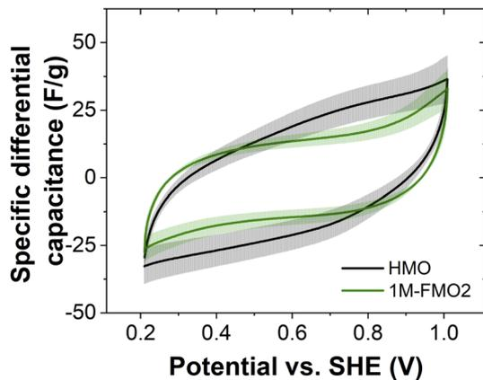
Fig. 2 Averaged specific differential capacitance of 2D  $\text{MnO}_x$  nanosheets (HMO) and nanocone-rich  $\text{Fe}_x\text{Mn}_{1-x}\text{O}_2$  (1M-FMO2) sample. The standard deviation was used to obtain the error bar reported in the plot.
