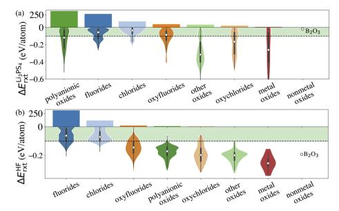
Fig. 3 Distribution of the reaction energy  $\Delta E_{rxt}$  with Li<sub>3</sub>PS<sub>4</sub> (a) and HF (b) for each category that pass chemical stability with the cathodes descriptor. The horizontal dash lines represent the limits of the descriptors. The histograms in (a) and (b) illustrate the numbers of compounds for each category that pass the descriptors.
