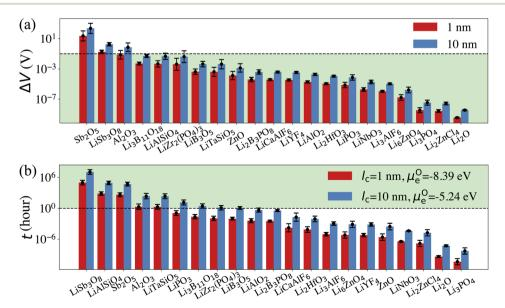
Fig. 5 (a) Calculated overpotentials ( $\Delta V$ ) for a current density of 0.044 mA cm<sup>-2</sup> across room temperature cathode coatings of  $l_c=1$  and 10 nm. The dashed line represents  $\Delta V=0.1$  V. (b) Calculated O<sup>2-</sup> diffusion time t in the selected compounds assuming an r=1  $\mu$ m primary particle and an  $l_s=2$  nm surface rocksalt phase. The dashed line represents t=1 h.
