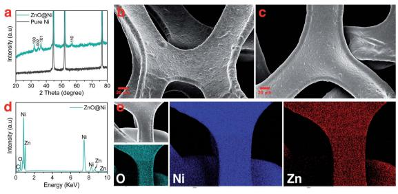
Fig. 1 Characterization of ZnO-coated nickel foam: (a) XRD pattern of pure Ni and ZnO-coated Ni foam, SEM image of (b) Ni foam and (c) ZnO-coated Ni, (d) EDS analysis of ZnO-coated Ni, and (e) SEM image and the corresponding elemental mapping of the ZnO-coated Ni sample.
