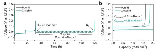
Fig. 5 Electrochemical performance: (a) Li plating-stripping voltage profile to calculate the average CE at 0.5 mA cm<sup>-2</sup> and (b) voltage profile of the last Li stripping from Ni and ZnO-coated Ni electrodes showing remaining capacity after 20 cycles of Li stripping/plating.
