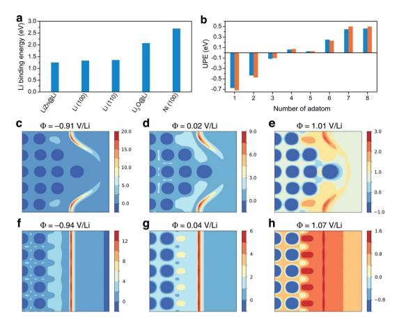
Fig. 3 Theoretical study: (a) Li binding energy computed for LiZn@Li (100), Li (100), Li (110), Li (20@Li (100), and Ni (100) surfaces. (b) Underneath plating energy computed on LiZn@Li (100), for different numbers of adatom. (c)–(e) and (f)–(h) Electrostatic potential computed for different potential values and projected on the [200] plane of the calculation cell, with and without the Li tip, respectively, as provided in Fig. S7.† Values are given in volt.
