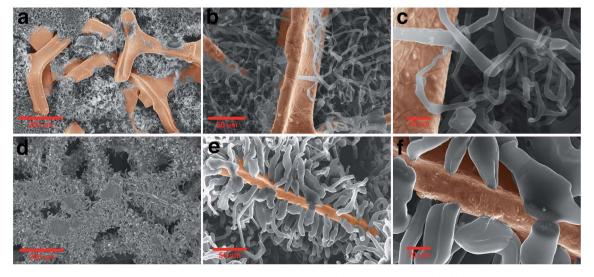
Fig. 4 Morphology evolution of the Li dendrite: comparing the SEM image of (a) – (c) pure nickel and (d) – (f) ZnO-coated Ni foam electrodes after growth of dendrite in different magnifications.
