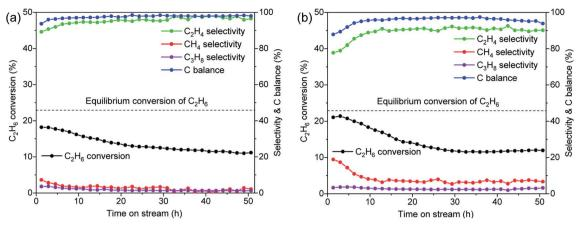
Fig. 8 Catalytic performances of (a) 0.5Co@MFI and (b) 1.3Co@MFI catalysts at 7.5 bar pressure. Reaction conditions: 50 mg catalyst, pretreatment by  $10\% \text{ H}_2/\text{N}_2$  for 30 min,  $20\% \text{ C}_2\text{H}_6/\text{N}_2$ , 5 mL min<sup>-1</sup>,  $650\% \text{C}_2$ .
