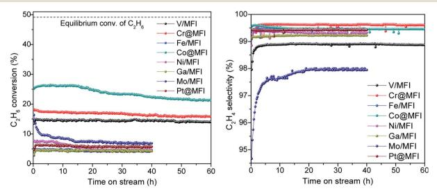
Fig. 1 EDH activities of different metal catalysts. Reaction conditions: 100 mg catalyst, pretreatment by 10%  $H_2/N_2$  for 30 min, 20%  $C_2H_6/N_2$ , 10 mL min<sup>-1</sup>, 1 bar, 650 °C.
