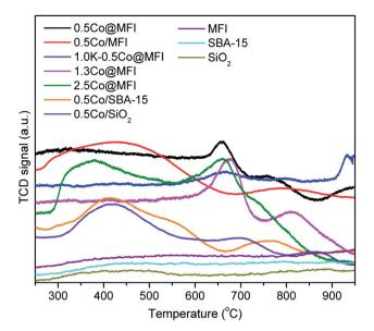
Fig. 4 H<sub>2</sub>-TPR profiles of different Co-based catalysts and bare supports
