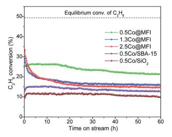
Fig. 5 Effect of Co loading and catalyst support on the EDH activities of different Co catalysts. Reaction conditions: 100 mg catalyst. pretreatment by 10%  $H_2/N_2$  for 30 min, 20%  $C_2H_6/N_2$ , 10 mL min<sup>-1</sup>, 1 bar, 650 °C.
