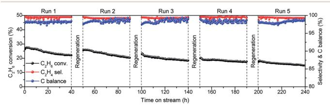
Fig. 7 Recycling experiment with 0.5Co@MFI catalyst. Reaction conditions: 100 mg catalyst, pretreatment by 10%  $H_2/N_2$  for 30 min, 20%  $C_2H_6/N_2$ , 10 mL min<sup>-1</sup>, 1 bar, 650 °C.
