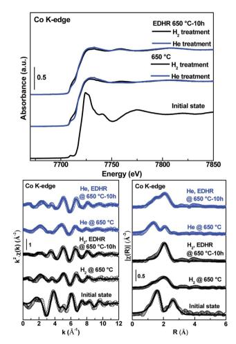
Fig. 9 Evolution of Co K-edge XANES spectra (top) of 0.5Co@MFI at the initial state, after pretreatment, and after EDHR.  $k^2$  weighed EXAFS spectra (bottom left) and FTs (bottom right) of 0.5Co@MFI at the initial state, after  $H_2$  pretreatment, and after EDHR.
