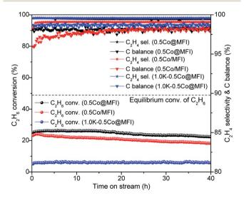
Fig. 6 EDH performances of 0.5Co@MFI, 0.5Co/MFI, and 1.0K-0.5Co@MFI at 1 bar pressure. Reaction conditions: 100 mg catalyst, pretreatment by 10%  $H_2/N_2$  for 30 min, 20%  $C_2H_6/N_2$ , 10 mL min<sup>-1</sup> 650 °C.
