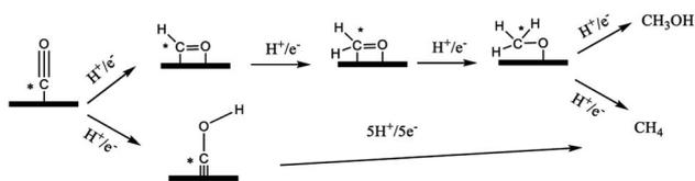
Fig. 6 ECR catalytic pathways for deeply reduced C<sub>1</sub> products at the catalytic interface.
