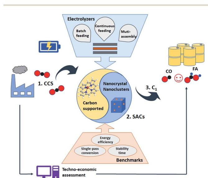
Fig. 1 Schematic of the whole industrial ECR process: the regulation of SACs is the crucial link for transferring CO<sub>2</sub> from carbon capture and storage (CCS) to C<sub>1</sub> products. Multi-assembly electrolyzer scales up the yield of C<sub>1</sub>. Through techno-economic assessment of the full lifecycle, the ECR performance satisfies the benchmarks, indicating that SACs are suitable for scaled-up use in industry.
